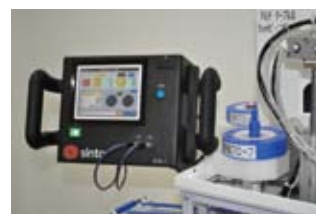
PSMX-I, new X-ray stress measuring device
