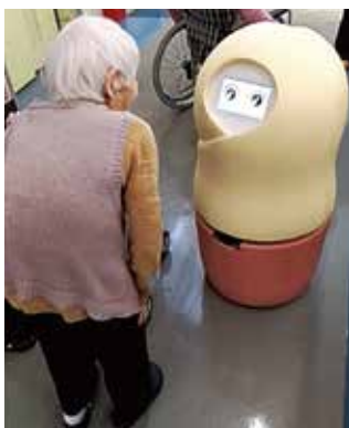
Monitoring robot Kurumi for nursing care facilities
