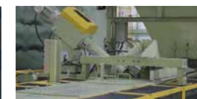
Sand property control equipment
