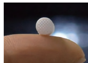
Sample with a minimum hole diameter of 0.3 mm
