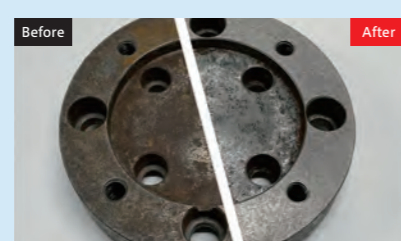
Rust removal using laser cleaning, before (left) and after (right) treatment
