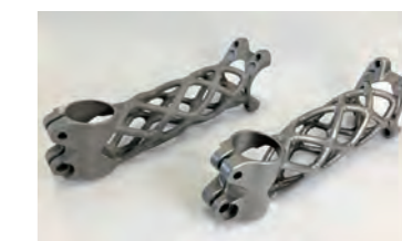
Metal AM sample before (left) and after (right) surface treatment
