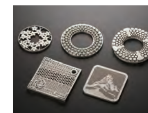
Metal samples from the Exentis 3D printer
