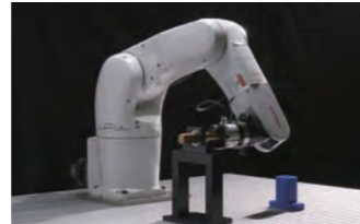
Shaft fitting by a robot equipped with ZYXer
