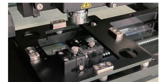
Measuring the dimensions of an MT ferrule (a connector component for optical fibers)
