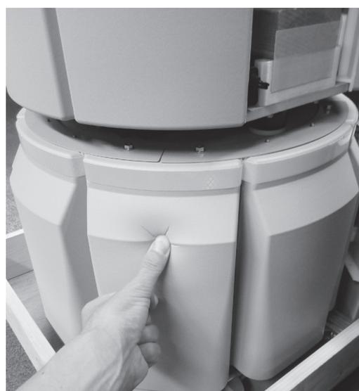
Fig. 6 Flexible exterior with contact detection function
