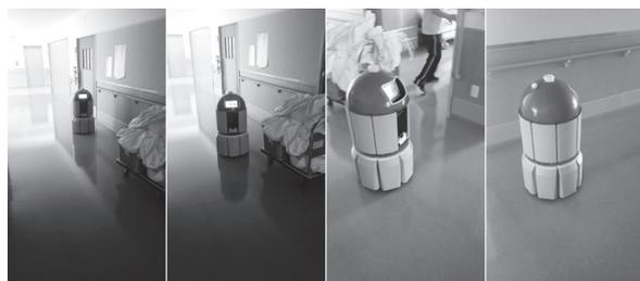
Fig. 4 A robot that automatically avoids dolly
