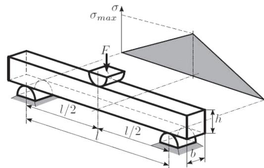
Fig. 1(a) Schematic for 3-point bend test<sup>8</sup>
