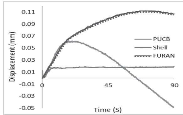
Fig. 3 Longitudinal displacement of various sand binder system
