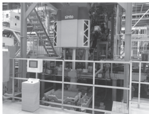
Fig. 1 Tight Flask Molding Machine ACEX.
